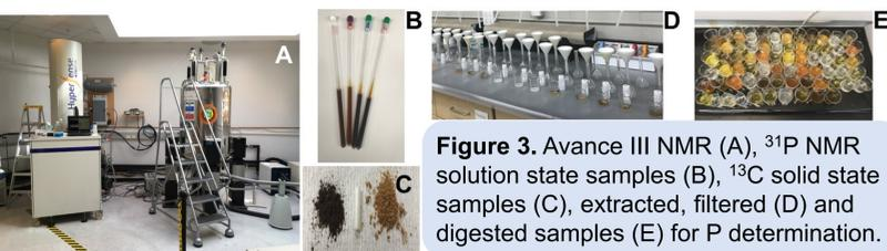
Figure 3. Avance III NMR (A), <sup>31</sup>P NMR solution state samples (B), <sup>13</sup>C solid state samples (C), extracted, filtered (D) and digested samples (E) for P determination.
